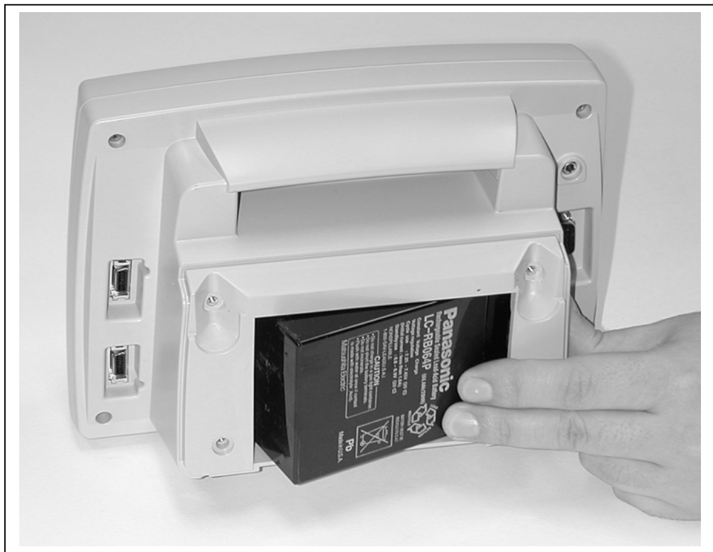
Figure 4-2. Monitor Tilted, Battery Removal in Process
